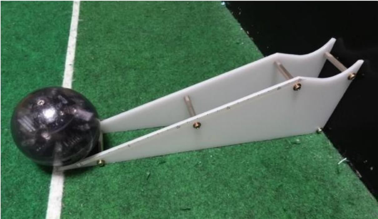
Fig. 1. Kicker Power Measuring Device
